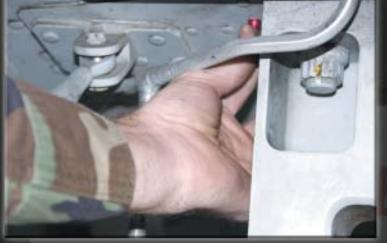
Staff Sgt. Micah Gaches checks the rivets on a 442nd Fighter Wing A-10 as part of a mandatory inspection across the Air Force's A-10 fleet to look for very small cracks in certain airplanes.
