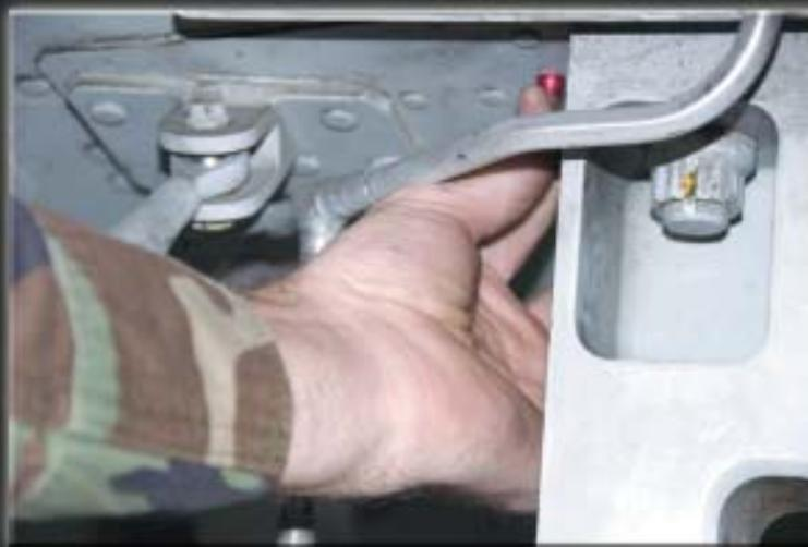
*Staff Sgt. Micah Gaches checks the rivets on a 442nd Fighter Wing A-10 as part of a mandatory inspection across the Air Force's A-10 fleet to look for very small cracks in certain airplanes.*
